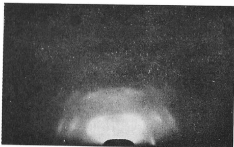
Fig. 4. Electron diffraction pattern of textured \beta -tantalum condensed on fused quartz at T = 400^\circ\text{C}
